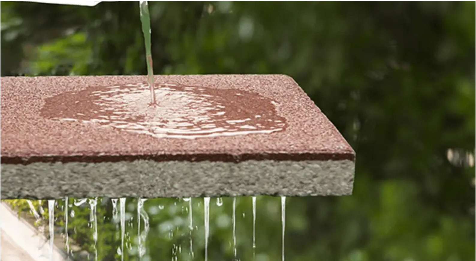
Permeability demonstration image
